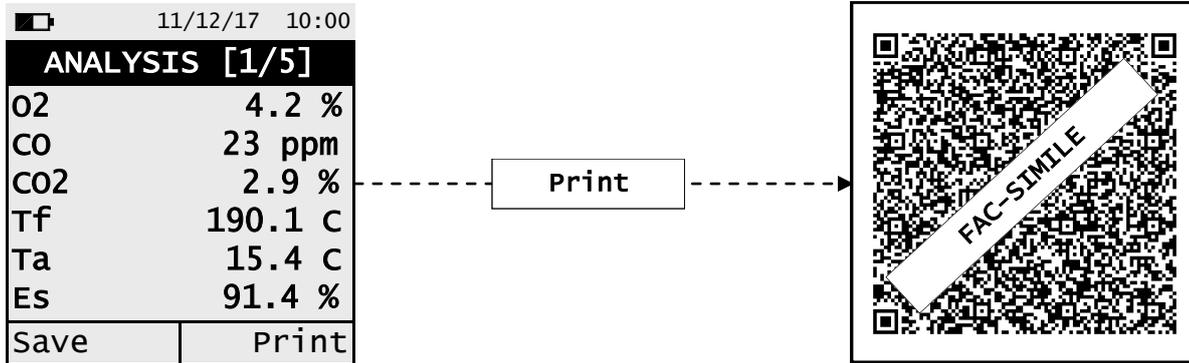
SCAN THE QR CODE USING SEITRON APP “SMARTFLUE LITE MOBILE”, TO DOWNLOAD THE ACQUIRED DATA.
